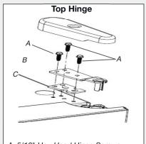
A. 5/16" Hex-Head Hinge Screws B. Top Hinge C. Spacer In case your refrigerator has electronic control on the door disconnect the cables and connect them on the other side
