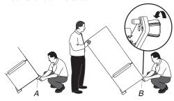
A. Remove runner. B. Install leveler.
